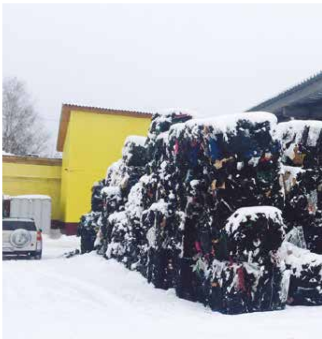
Pic. 2 Reworked polyethylene raw materials can be used for the production of packaging, roofing materials, cans and other goods. They cannot be used for the production of pressure pipes! (The picture was taken at Noginsk Plant of polymer materials)
